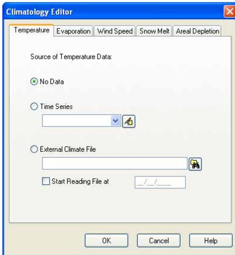
The Temperature page of the Climatology Editor dialog is used to specify the source of temperature data used for snowmelt computations. There are three choices available:
