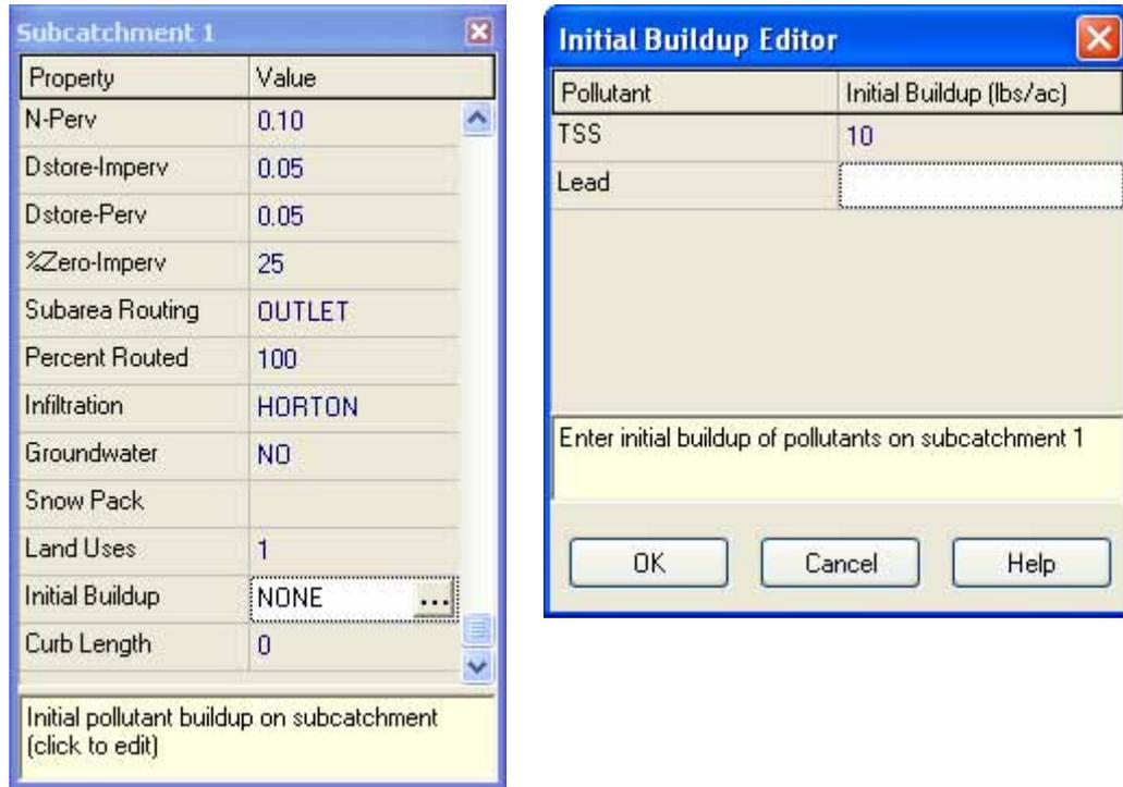
If a non-zero value is specified for the initial buildup of a pollutant, it will override any initial buildup computed from the Antecedent Dry Days parameter specified on the Dates page of the Simulation Options dialog.
