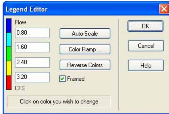
The Legend Editor is used to set numerical ranges to which different colors are assigned for viewing a particular parameter on the network map. It works as follows:
