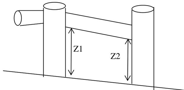
These offsets are expressed as a relative distance above the node invert if the **LINK\_OFFSETS** option is set to **DEPTH** (the default) or as an absolute elevation if it is set to **ELEVATION**.
