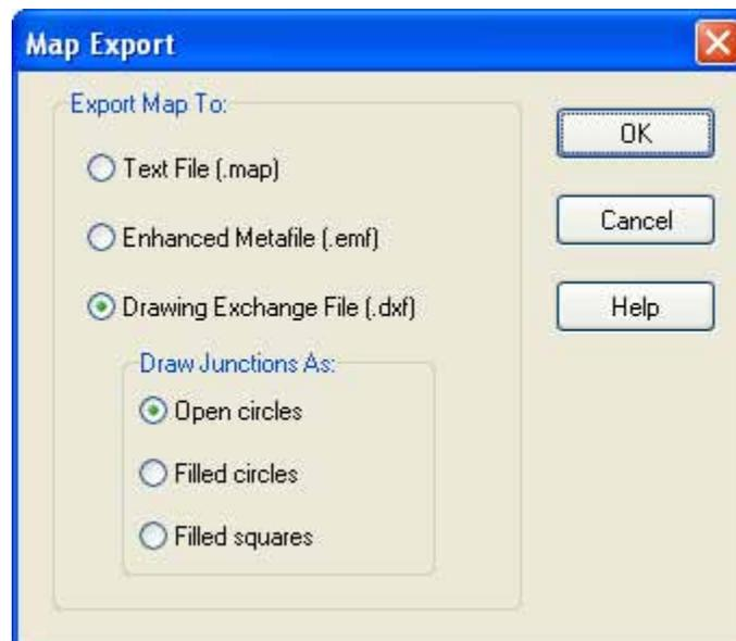
If you select DXF format, you have a choice of how nodes will be represented in the DXF file. They can be drawn as filled circles, as open circles, or as filled squares. Not all DXF readers can recognize the format used in the DXF file to draw a filled circle. Also note that map annotation, such as node and link ID labels will not be exported, but map label objects will be.
