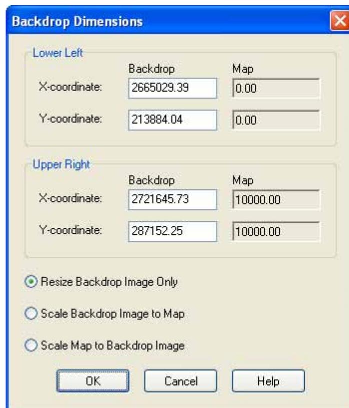
The dialog lets you manually enter the X,Y coordinates of the backdrop's lower left and upper right corners. The Study Area Map's dimensions are also displayed for reference. While the dialog is visible you can view map coordinates by moving the mouse over the map window and noting the X,Y values displayed in SWMM's Status Panel (at the bottom of the main window).
