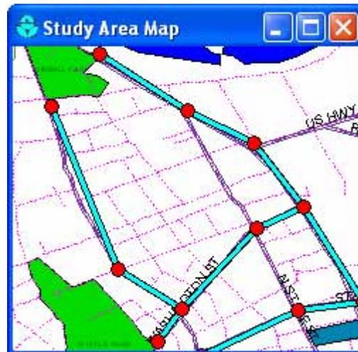
The backdrop image must be a Windows metafile, bitmap, or JPEG image created outside of SWMM. Once imported, its features cannot be edited, although its scale and viewing area will change as the map window is zoomed and panned. For this reason metafiles work better than bitmaps or JPEGs since they will not lose resolution when re-scaled. Most CAD and GIS programs have the ability to save their drawings and maps as metafiles.
